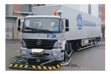
A tractor trailer leaves the loading ramp and starts to travel across the company's premises without a driver sitting behind the steering wheel. What sounds like science fiction has long been reality in many factories. Automated guided vehicles like fork lifts, freight platforms with own transmission or trucks are used to move goods from point A to B wherever rail vehicles or conveyor lines are too expensive, too complicated or too inflexible.
