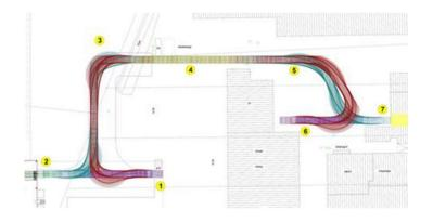
The final dimensions of the path are determined using the vehicle's parameters. "By ensuring that the trajectory takes these parameters into account and that the curve radii and steering speeds are selected accordingly, it is possible to make sure that the vehicle can manage all curves as well," states the software developer Malz. In doing so, the travel path of a trailer is also taken
