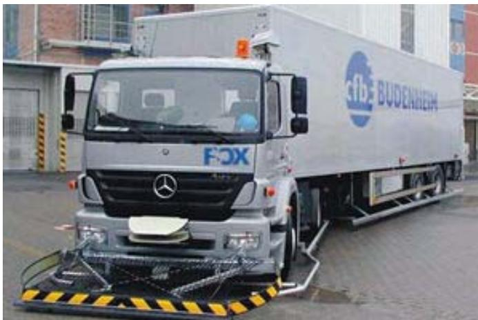
A tractor trailer leaves the loading ramp and starts to travel across the company's premises without a driver sitting behind the steering wheel. What sounds like science fiction has long been reality in many factories. Automated guided vehicles like fork lifts, freight platforms with own transmission or trucks are used to move
